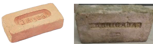
Figure 2: Red clay brick (left) and refractory brick (right)
