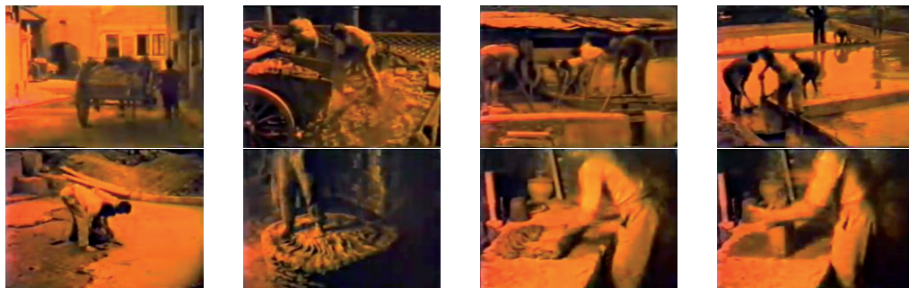
Figure 1: Clay and paste preparation. Video print screen (Matos, 2014)
