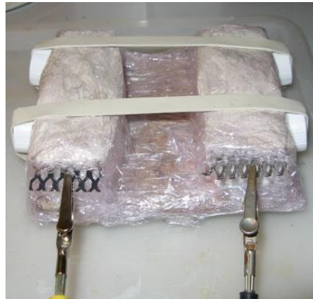
Figure 3: Experimental setup for desalination of single tile
