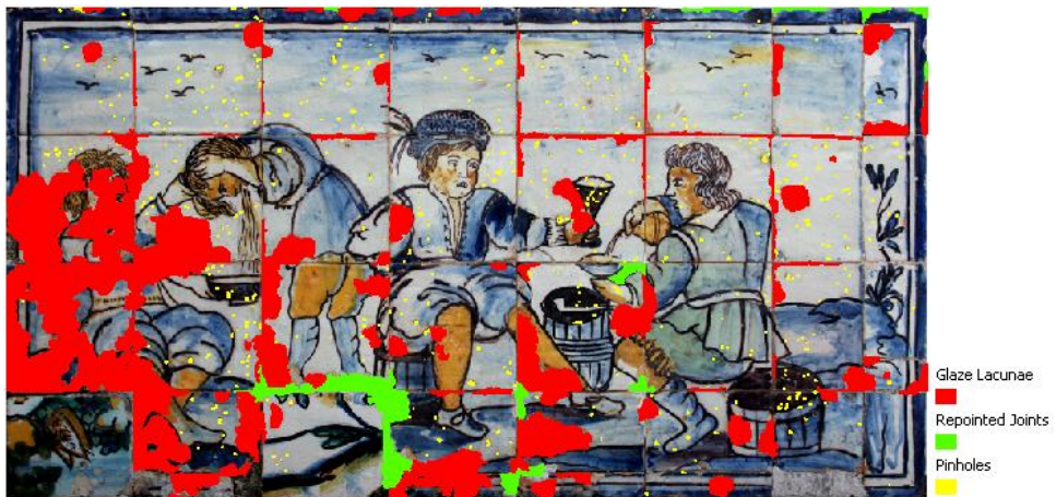
Figure 4 – Pathologies map produced with OBIA
