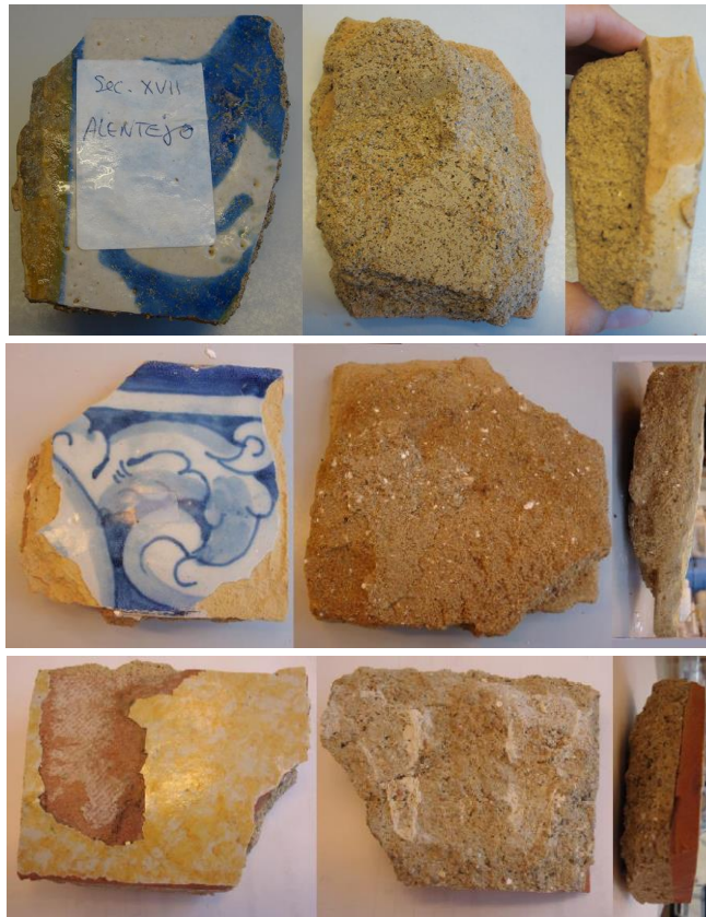
Figure 5: experimental tiles with mortar. (a) 17 th century tile from the Alentejo Region (b) 18 th century tile from Palacio Centeno, Lisbon (c) and 20 th century tile of unknown origin.
