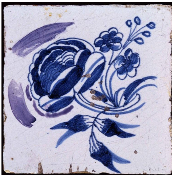
Figure 1. Two areas of a non-metameric pigment retouching recipe which match the blue of the tile design perfectly in daylight but, in the lighting of this image, are very discordant
