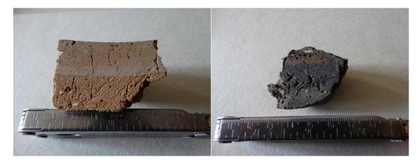
Figure 1 – left: Fragment of a casting mold from Olympia (Oly 1, G 1685) indicating construction of different layers; right: fragment of a crucible from Athens (Ker 2, G 2926)
