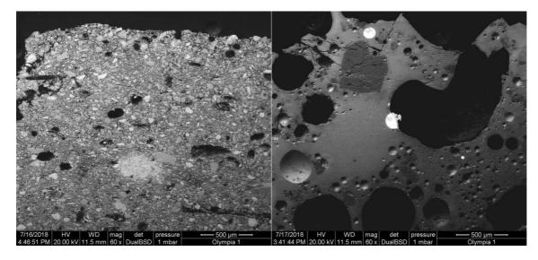
Figure 3 – left: SEM micrograph in backscattering mode of a section of a casting mold from Olympia (Oly 1, G 1685) presenting the characteristic pore structure of the internal layer; right: SEM micrograph in backscattering mode of a section of a crucible from Athens (Ker 2, G 2926) presenting the slagged internal surface with large bloating pores and prills of the processed metals.
