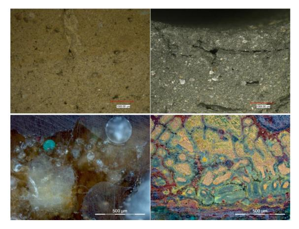
Figure 2 – top left: Micrograph of a casting mold from Olympia (Oly 1, G 1685) indicating the layered construction with different clay pastes; top right: Micrograph of a casting mold from Athens (Ker 1, G 2924) presenting large voids and cracks parallel to the surface; bottom left: Micrograph of a fragment of a crucible from Athens (Ker 2, G 2926) presenting a copper prill; bottom right: Micrograph of a fragment of a crucible from Olympia (Oly 5, G 1682) presenting a copper inclusion.
