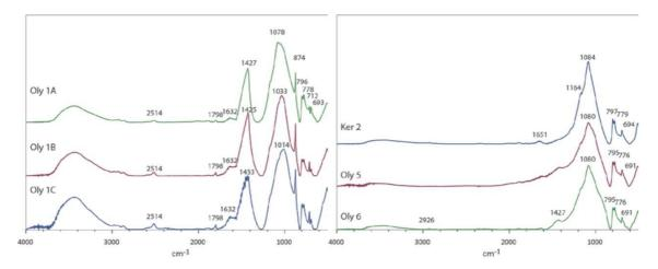
Figure 4 – left: FTIR spectra of the three ceramic layers of a casting mold from Olympia (Oly 1, G 1685); right: FTIR spectra of a crucible from Athens (Ker 2, G 2926) and two crucibles from Olympia (Oly 5, G 1682: Oly 6, G 1678).
